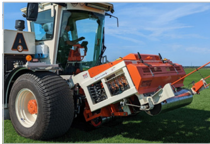
24-in cutting heads with adjustable down pressure
