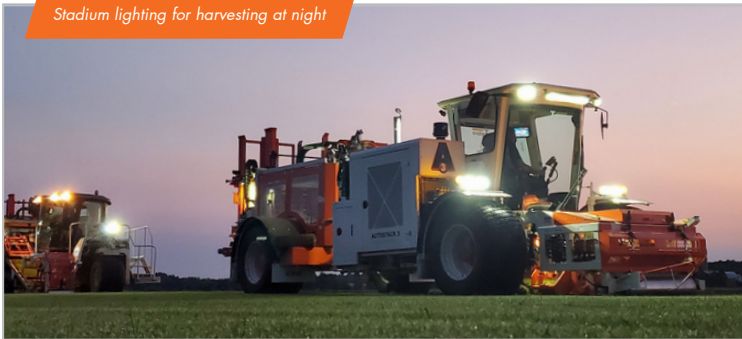
24-in cutting heads with adjustable down pressure
