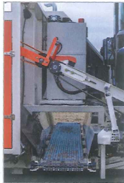
Cross-conveyor scrap dump - puts scrap out of the way
