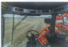
Cab rotates 90° into harvesting position for excellent visibility and operator comfort
