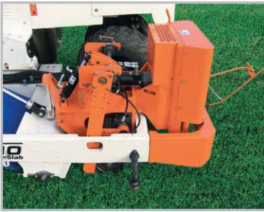
Floating cutting head with adjustable-down pressure
